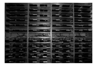
many processes can profitably be squeezed together. The examples given below were run on LACAL's cluster of more than 215 PS3s (see picture), i.e., about 1300 SPUs.
